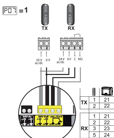
**Photoelectric cells - with autotest**
