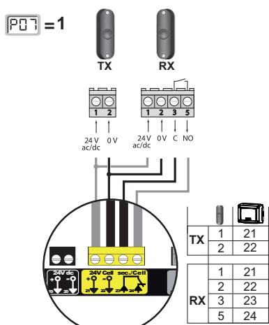
**Fotoseller - otomatik test var**
